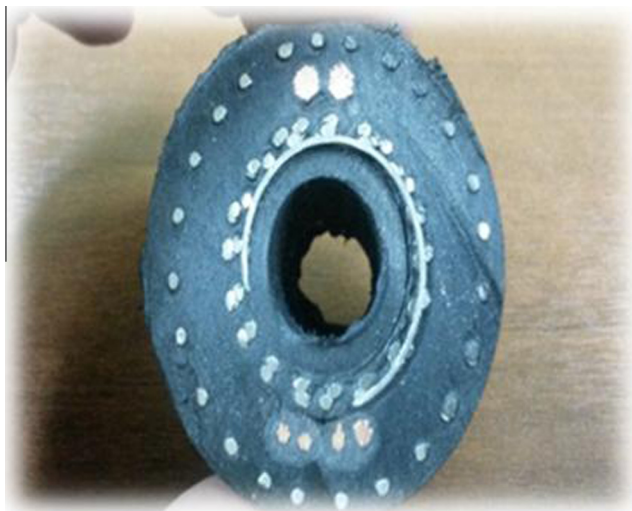
Fig. 3. Cross-section of the cable with hydraulic channel and power and signal cores.
