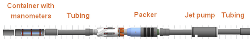
Fig. 7. Configuration of downhole equipment during treatment.
