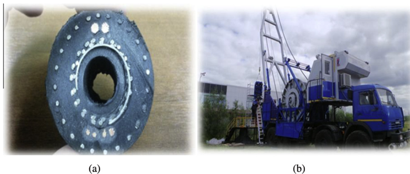
Fig. 4. Equipment used for selective ultrasonic treatment of horizontal wells: (a) cable (b) “mini coiled tubing” wireline truck.
