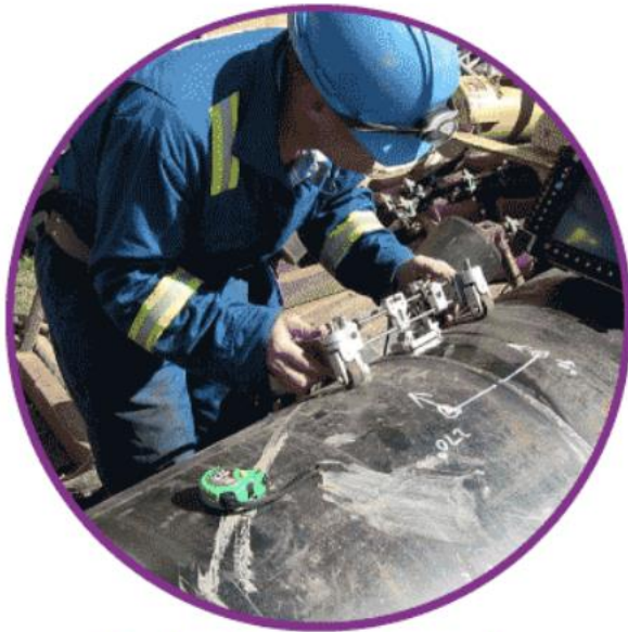
Fig.3.12 Cracks detection in metallic components using ultrasound
