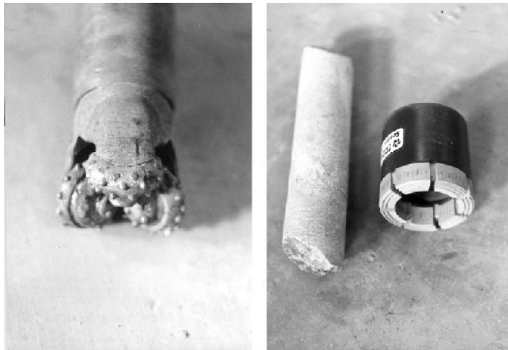
Figure 4.6 Three-cone roller bit (left). Rock coring bit and segment of rock core (right).
