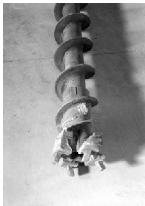
Figure 4.4 Hollow-stem auger with cutting bits at the bottom.
