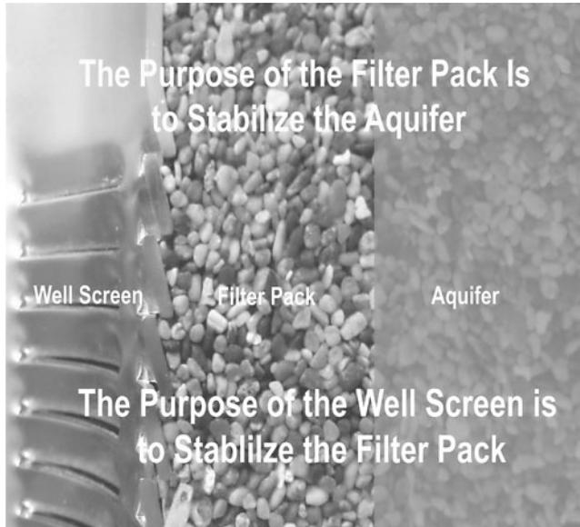
Fig. 4-16. Fundamental principle of well design and development
