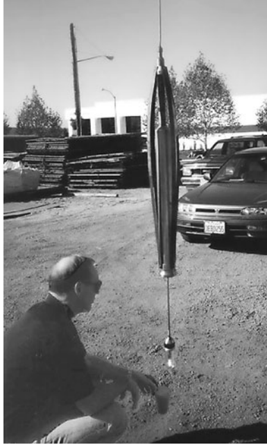
Fig. 4-24. Downhole video survey camera
