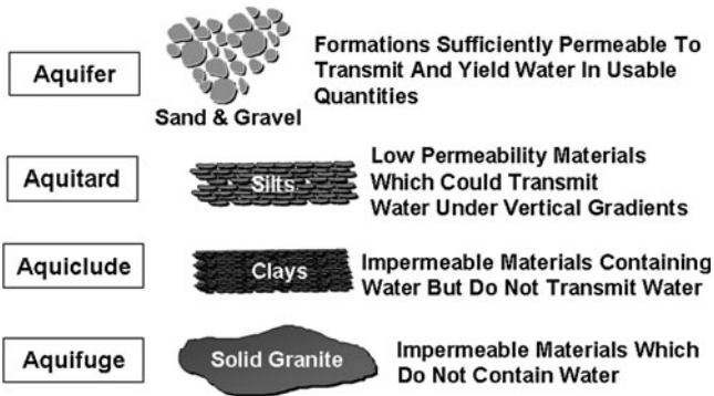
Fig. 1-4. Aquifer, aquitard, aquiclude, and aquifuge Source: Courtesy of Dennis E. Williams, Geoscience Support Services, Inc., Claremont, CA
