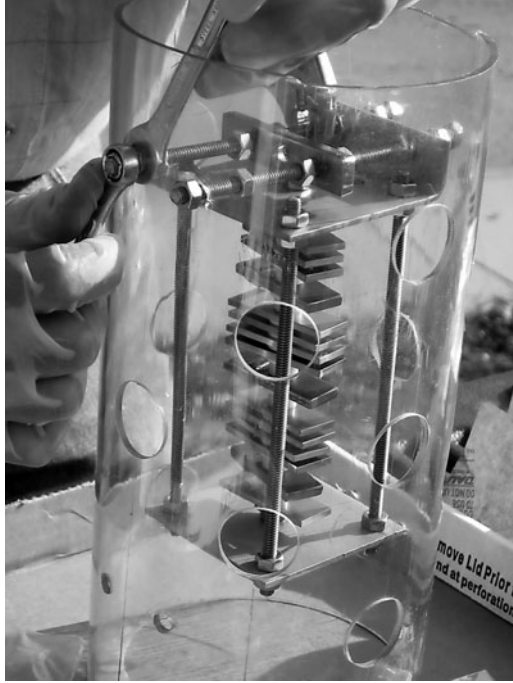
Fig. 5-3. Installing the test coupons in the coupon holder Source: Courtesy: Dennis E. Williams, Goescience Support Services, Inc., Claremont, CA; reproduced with permission from City of Ontario, CA
