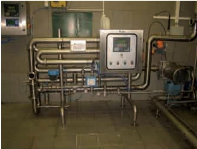
Equipment diluting "beer concentrate" to the required degree - HGB Photo: Author's archive
