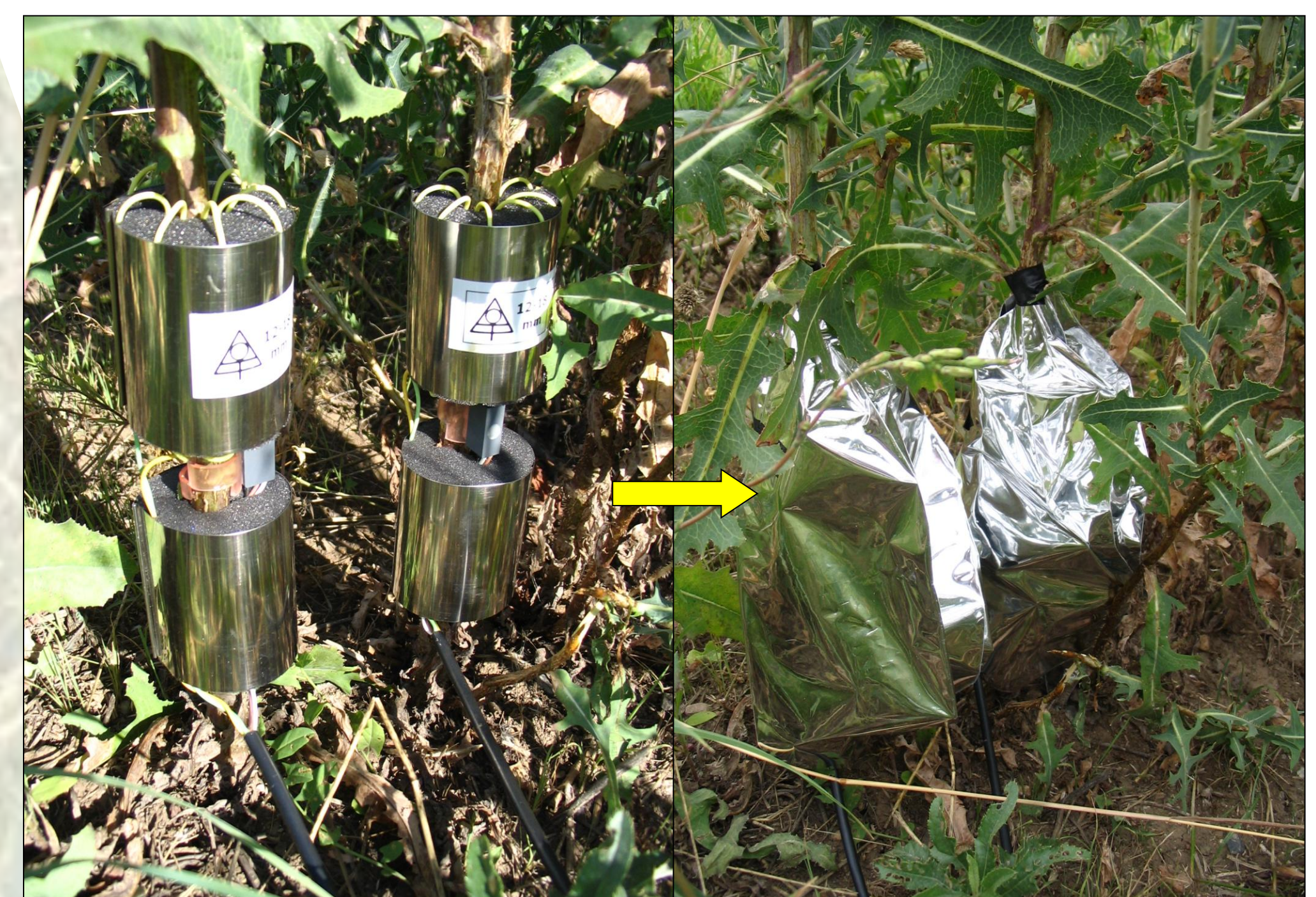
Installation of sap-flow meter T 4.2
