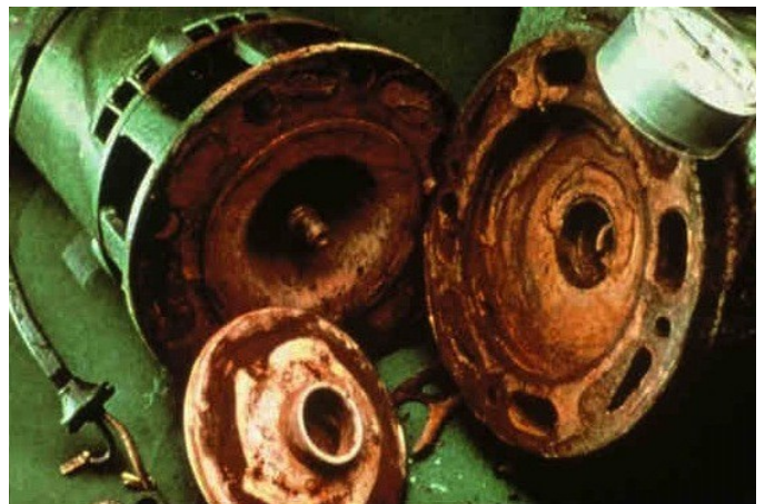
Abrasion caused by pumping sand.
