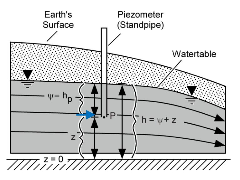
A piezometer measures the hydraulic head at a point.
