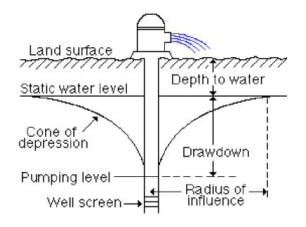
Details on the geometry of drawdown and the "cone of depression".
