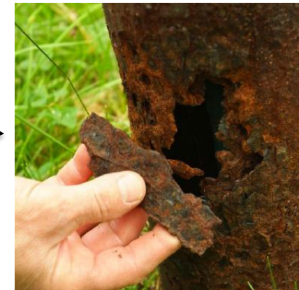
Holes in casing caused by corrosion
