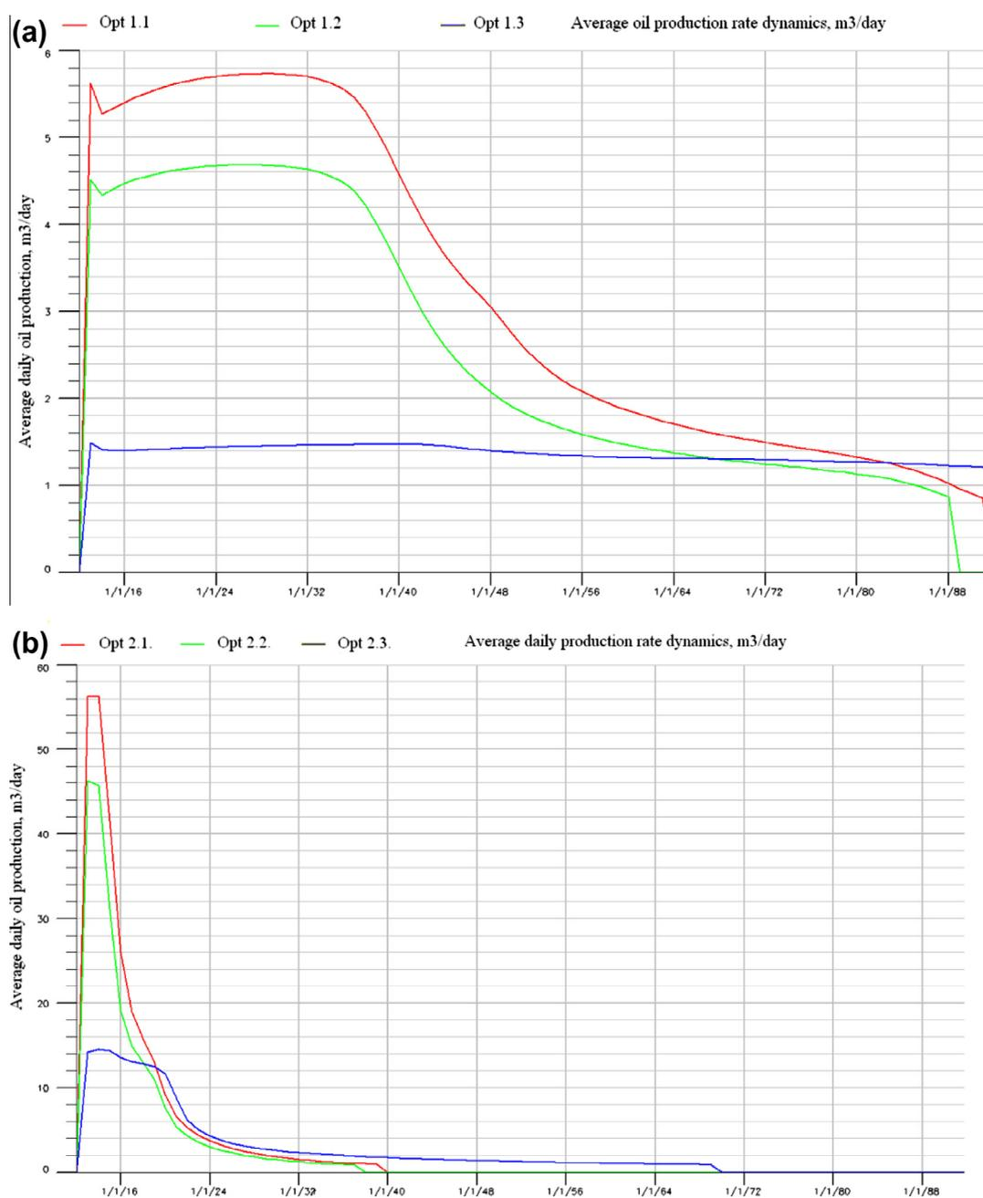
Fig. 5. Dynamics of average daily oil production for an area with permeability 13 mD (a) and 114 mD (b).
