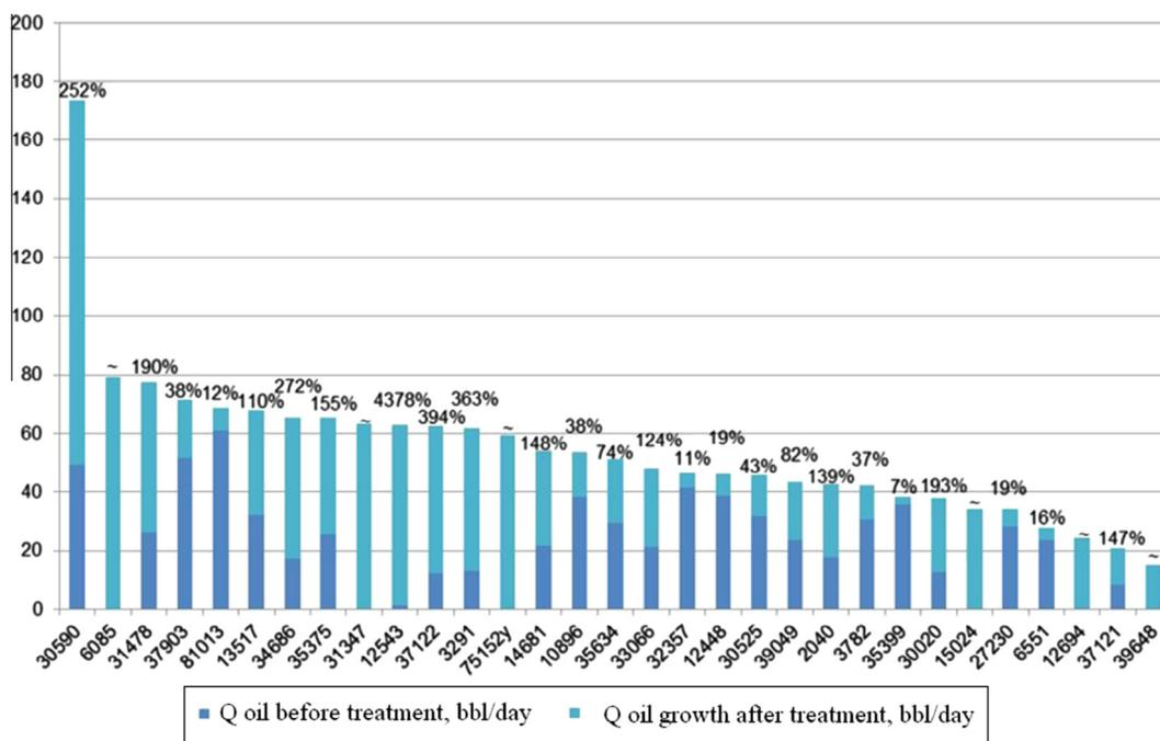
Fig. 3. Production changes after the ultrasonic treatment of the BHZ of wells in AB reservoirs.
