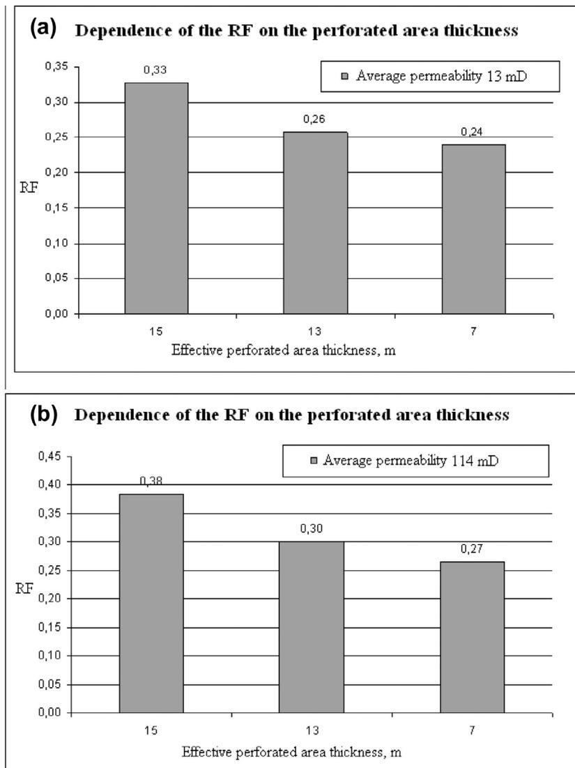
Fig. 6. Dependence of the recovery factor on the perforated area thickness for an area with permeability 13 mD (a) and 114 mD (b).
