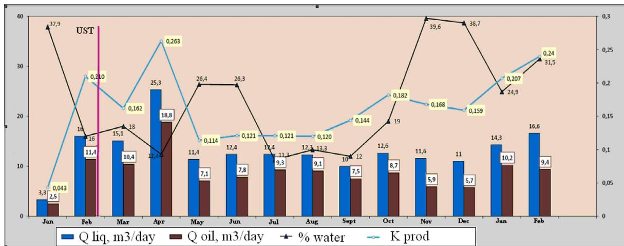
Fig. 2. Dynamics of flow rates before and after the ultrasonic treatment of well no. 34686:  $Q_{liq}$  – the daily production rate of fluid,  $Q_{oil}$  – the daily oil production rate, % water – percent water cut,  $K_{prod}$  – productivity coefficient.
