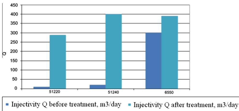
**Fig. 4.** Injectivity change of injection wells in BC reservoirs after combined ultrasound and chemical treatment.
