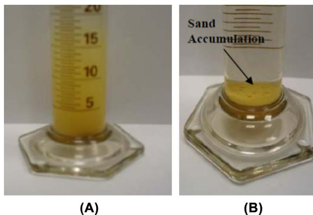
**Figure 11** Images showing the sand production: (A) while waterflooding and (B) after sand grains have settled at the bottom of the glass cylinder.
