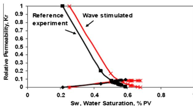
**Figure 6** Effect of wave stimulation on the water/oil relative permeability in vertical corefloods.
