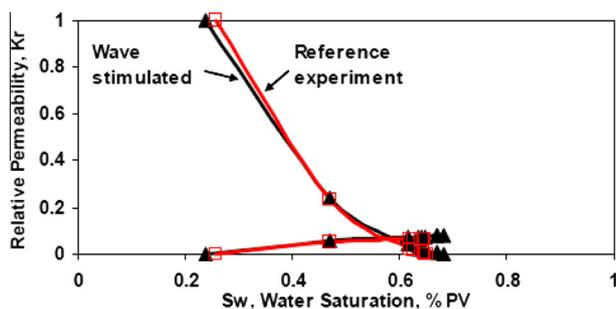
**Figure 2** Behavior of water/oil relative permeability in absence and presence of wave stimulation at OOIP.
