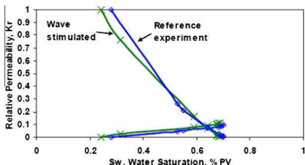
**Figure 5** Water/oil relative permeability in cores with higher initial permeability.
