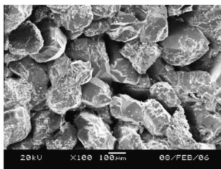
**Figure 12** SEM photo showing the general texture of the core sample having a compressive strength of higher than 150 psi after wave stimulation.
