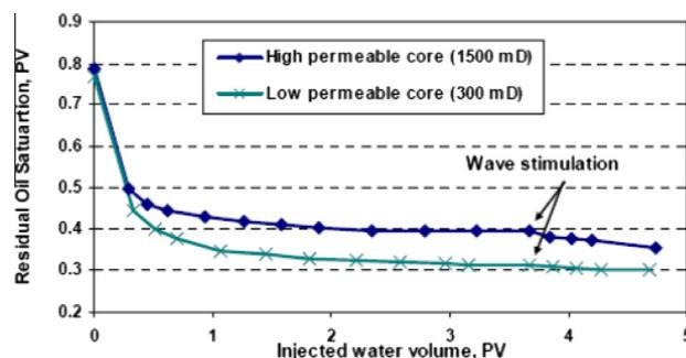
**Figure 9** Effect of wave stimulation on the oil recovery in high and low permeable core tests.
