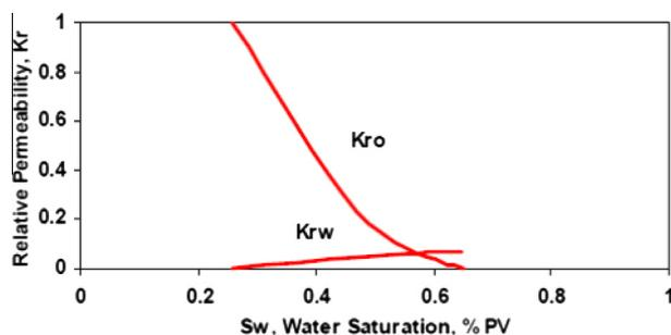
**Figure 1** Relative permeability curves to water and oil in the absence of wave stimulation as a reference experiment.
