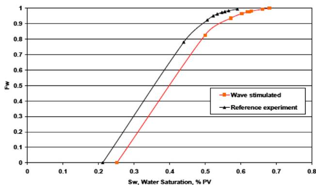
**Figure 7** Comparison of fractional flow curves for water in the presence and the absence of wave stimulation in vertical corefloods.
