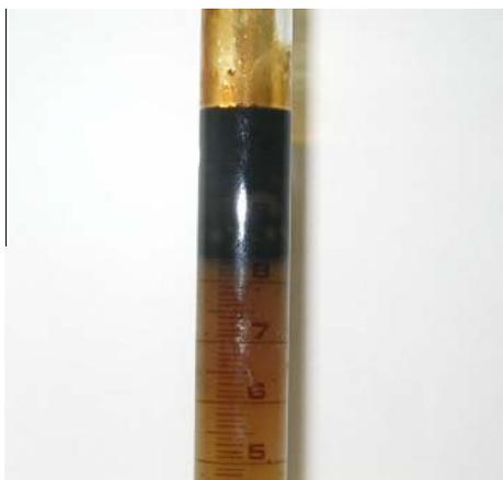
**Figure 10** Generated emulsion with low stability observed in the effluent.
