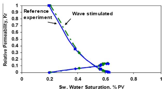
**Figure 8** Effect of wave stimulation on water/oil relative permeability on low permeable core samples.
