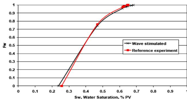
**Figure 3** Fractional flow curves of reference and wave stimulated experiments.
