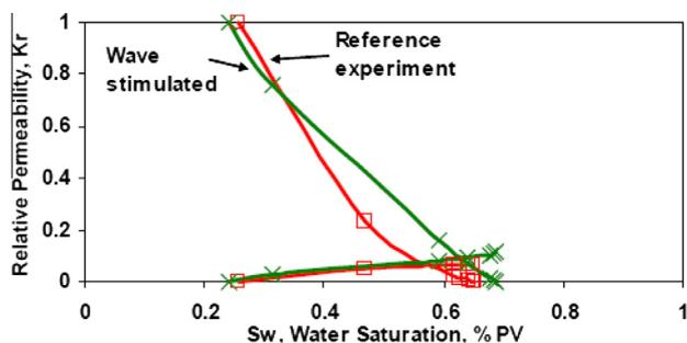
**Figure 4** Effect of wave stimulation on the water/oil relative permeability in high permeable core sample.
