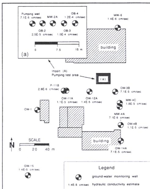
Fig. 1. Estimates of hydraulic conductivity using late-time slug-test data for the 13 monitoring wells and the pumping well at a ground-
