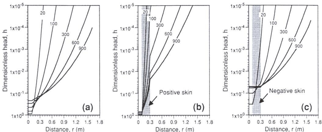
Fig. 3. Axisymmetric profile of dimensionless head across the tested well and formation at 20, 100, 300, 600, and 900 seconds: (a) in situ formation; (b) positive wellbore skin; and (c) negative wellbore skin. Patterned area indicates wellbore skin.
