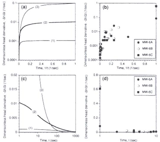
Fig. 6. Correlations of time versus dimensionless head derivative for the numerically simulated (a and c) and field-measured (b and d) slug-test data. Labels 1, 2, and 3 refer to, respectively, positive wellbore skin, undisturbed formation, and negative wellbore skin. MW-6A, MW-6B, and MW-6C are field slug tests at absent, complete, and extensive well development, respectively.
