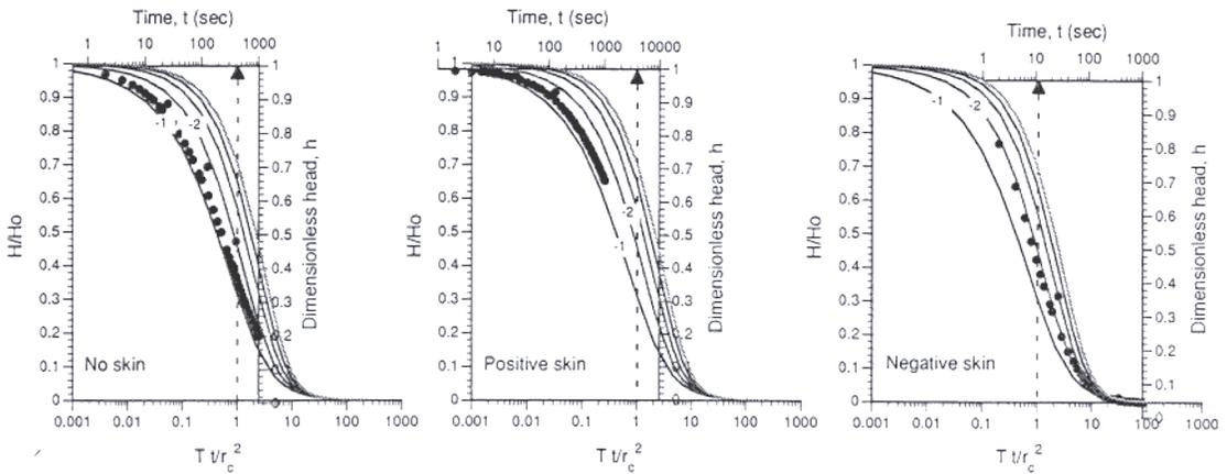
Fig. 5. Numerically simulated data in the semilog plot of dimensionless head versus the logarithm of time. Also shown are selected Cooper et al. (1967) type curves. Other labels in the diagram: -1 and -2 are the values of the parameter  $\log(\alpha)$ .
