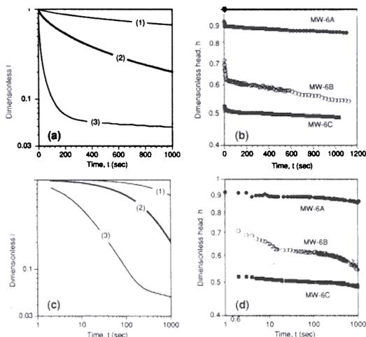
Fig. 4. Correlations between time and dimensionless head for the numerically simulated (a and c) and field-measured (b and d) slug-test data. Labels 1, 2, and 3 refer to, respectively, positive wellbore skin, undisturbed formation, and negative wellbore skin. MW-6A, MW-6B, and MW-6C are field slug tests at absent, complete, and extensive well development, respectively.
