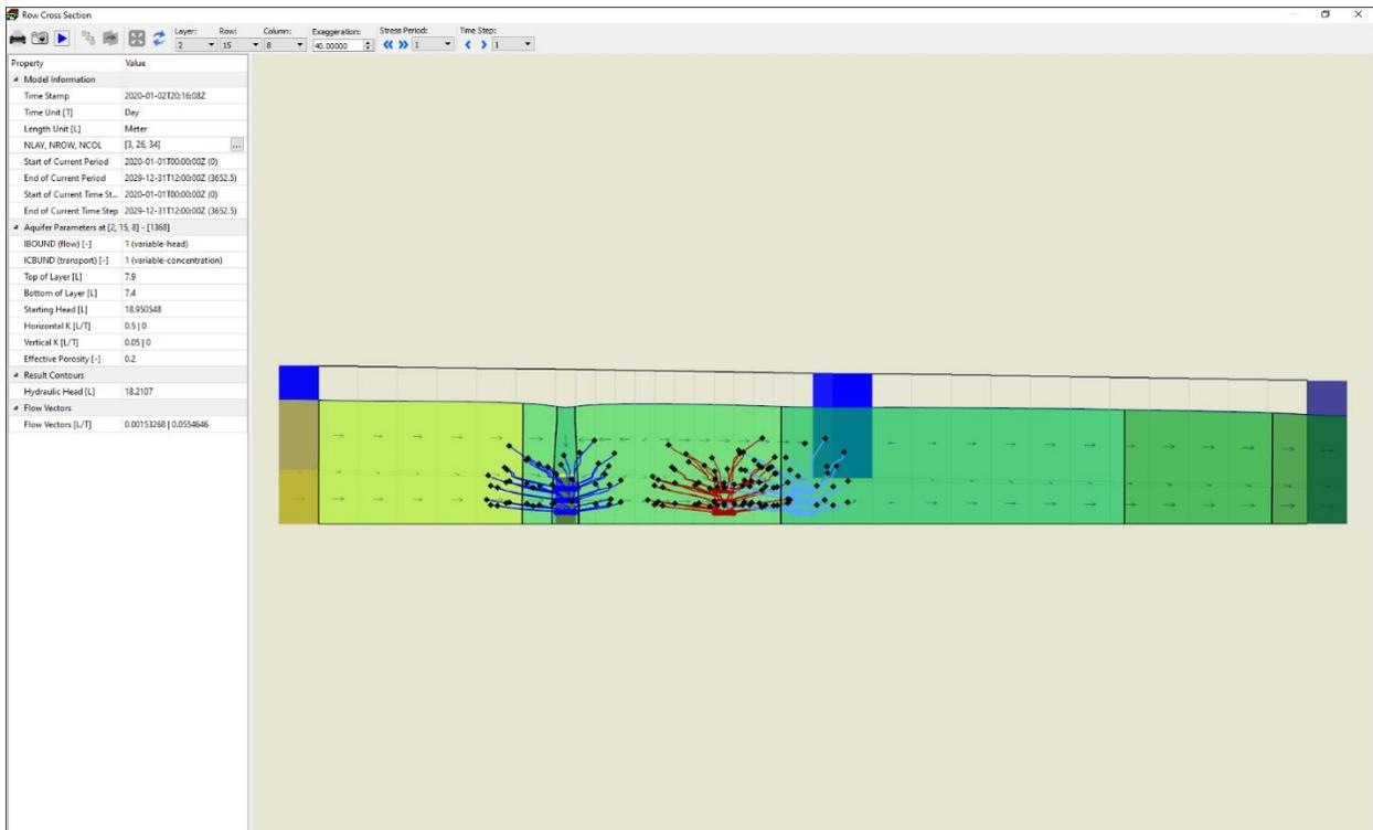
Figure 18. The projection of 10-year capture zones of pumping wells on the Row Cross Section window
