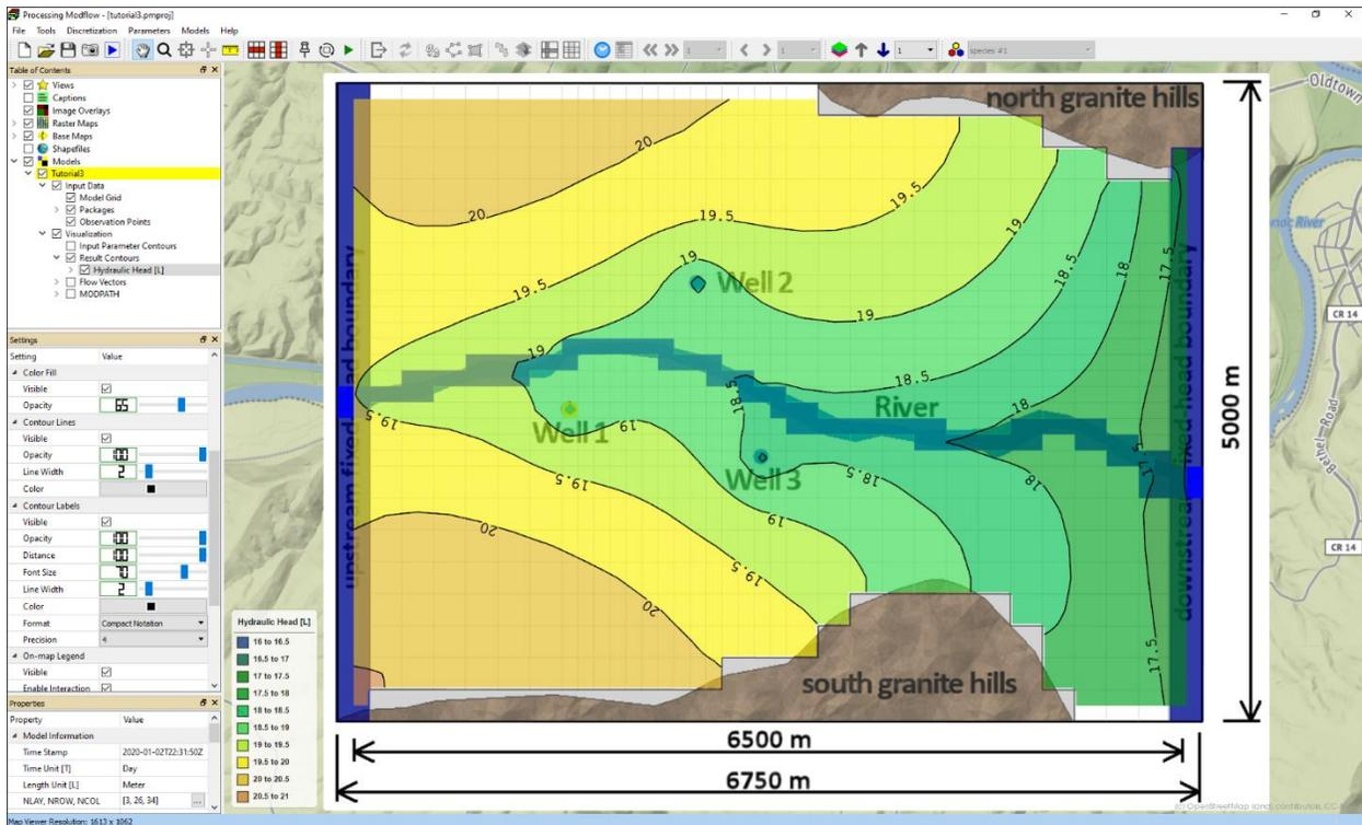
Figure 14. Color-filled hydraulic head contours of Layer 1
