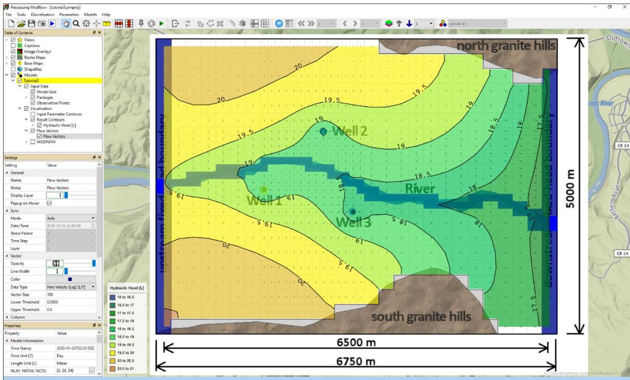
Figure 15. Flow vectors and color-filled hydraulic contours.
