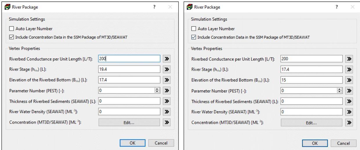
Figure 11. Parameters of upstream (left) and downstream vertex (right)
