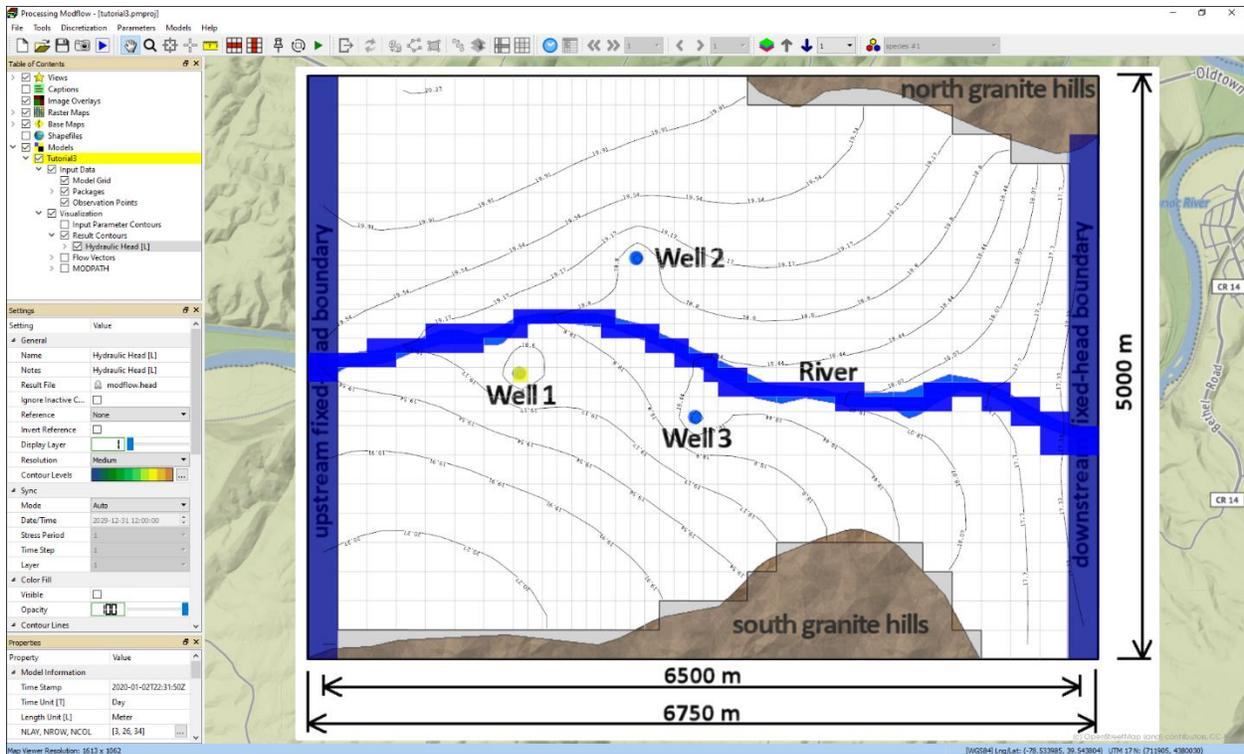
Figure 13. Hydraulic head contours of Layer 1
