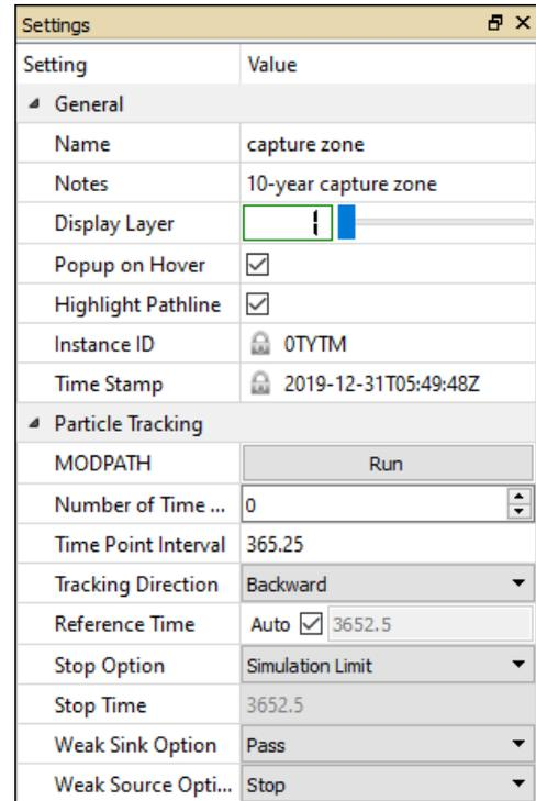
Figure 16. The Settings window of a MODPATH instance
