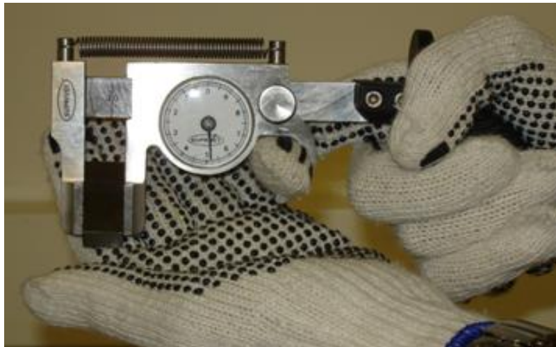
Fig. 2. Analog calliper during the calibration process
