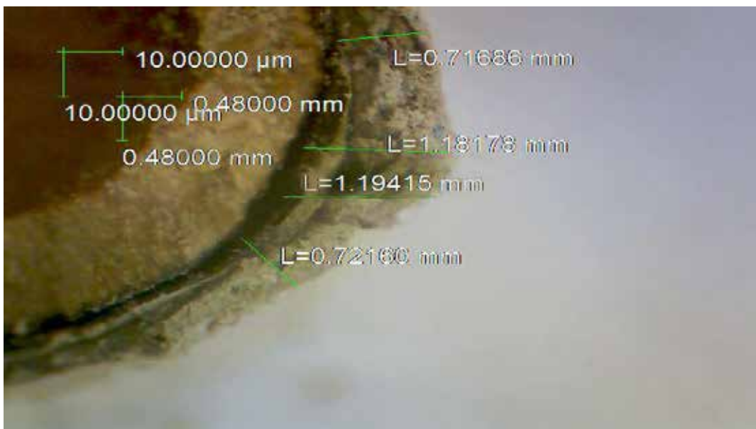
Figure 7 - Thickness of the layer of Korean cedar pine seed ( Pinus koraiensis Siebold et Zucc.) at the second stage of pelletizing (time - 2 + 6 min.)
