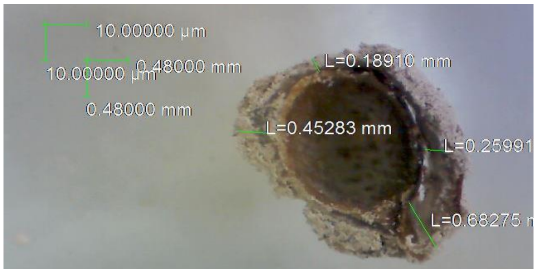
Figure 4 - Thickness of the layer of Scots pine seed ( Pinus silvestris L.) at the first stage of pelletizing (time - 7 minutes).
