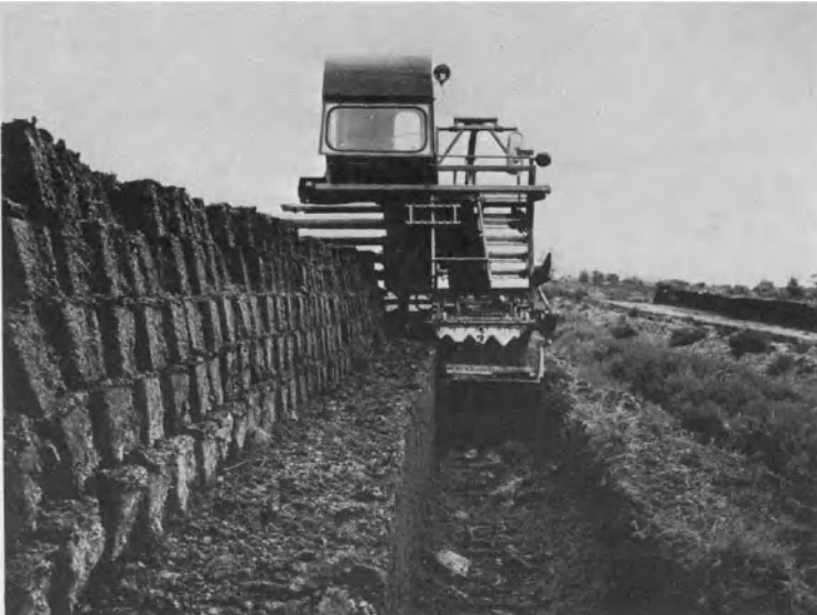
Figure 2.6 Peat harvesting with a sod-cutting machine (by permission of Bord Na Mona).
