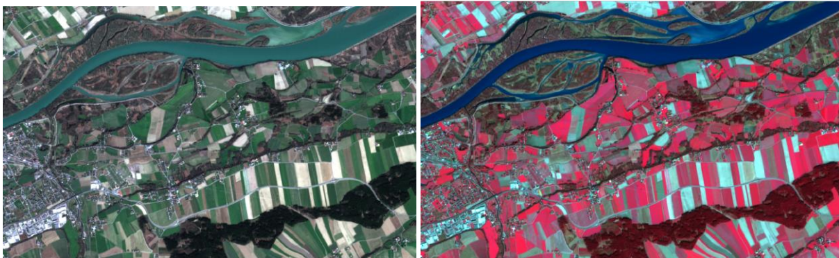
Figure 5. Various colour compositions: true colours (R-G-B) on the left and false colours (NIR-R-G) on the right.
