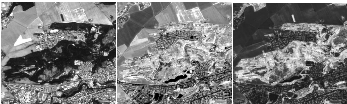
Figure 6. Sentinel-2A spectral band ratios – highlighting the differences in vegetation health status and unifying other types of landscape cover, the left image represents the red visible part of the spectrum (B4), infrared (B8) in the middle, the band ratio (B8/B4) on the right. In the red band, there is a high absorption of chlorophyll, while in the near-infrared zone there is a high reflectance of vegetation due to scattering in the lower part of the leaf.
